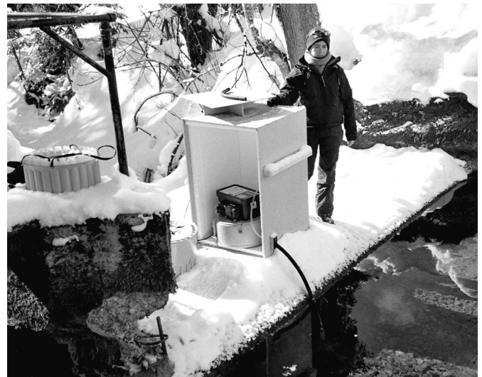
Fig. 2. Automatic sampler at the karst spring that drains the Hölloch cave in the Austro-German Alps (photo: N. Goldscheider). Due to temperatures down to -20^{\circ}\text{C} , the sampler was placed into a heated insulated box.
