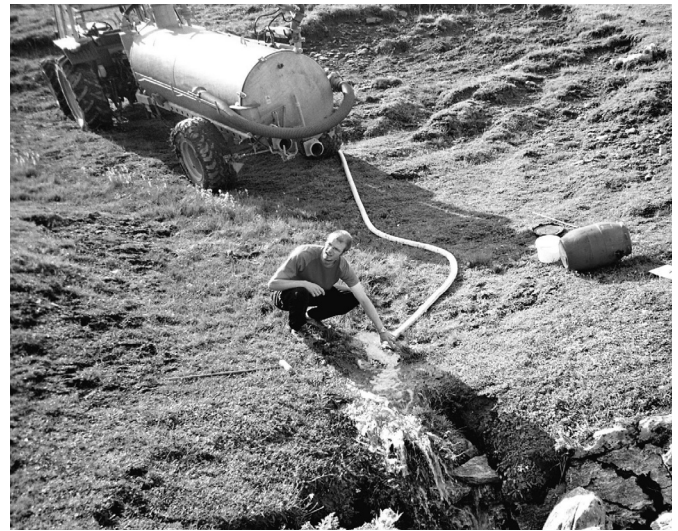
Fig. 1. Introduction of flushing water from a tank truck during and after the injection of a salt tracer into a shaft, Tsanfleuron glacier and karst aquifer system, Swiss Alps (photo: N. Goldscheider).
